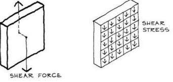
The distribution of shear stress cannot be deduced from the straightforward assumptions that were used for axial and bending stress. At the top and the bottom the shear stress must be zero, otherwise there would be vertical shear stresses on the surface of the beam, which is impossible. Mathematical analysis shows that for a rectangular beam the shear stress distribution has a curved shape, accurately described as parabolic distribution.
