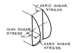
The maximum is at the middle of the beam, it is zero at the top and bottom and is constant across the width of the beam.
