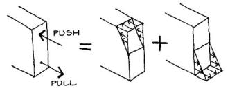
By varying the **depth** and therefore the lever arm, the size of the push and pull forces can be altered, which means the sizes of the stresses can be altered. This is only true if the width of the beam is not altered. The size of the stresses can also be altered by varying the width because this alters the area. Or the size of the stresses can be altered by varying both the depth and the width.
