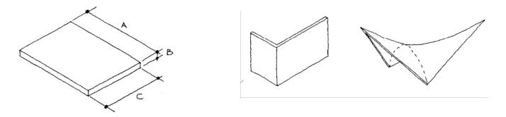
If two of the dimensions of the basic element, say B and C, are small compared with dimension A, then the element is a **one-dimensional element**. One-dimensional elements are used abundantly in nearly all buildings; examples are beams, bars, cables and columns.
