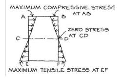
Using this information a stress distribution diagram can be drawn for the side view of the slice.
