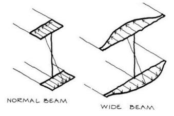
Axial forces and bending moments cause axial stresses, shear forces cause shear stresses. Because shear stresses resist vertical loads, it is to be expected that shear stresses act vertically. On the face of a beam slice, unlike the column, shear stresses (force per unit area) act in line with the face of the slice.
