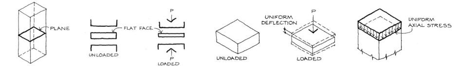
The uniform stress over the cross-section of an axially loaded column gives a very simple relationship between force and stress and this is:
