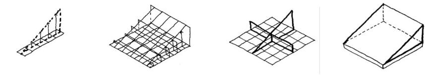
In general there is no restriction on how stresses vary across any cross-section of any structure, except that the sum of the stresses must be equal to the internal force acting at the section and that the internal force acts at the **center of gravity** of the stresses.
