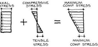
In this figure because the size of the axial compressive stress is bigger than the maximum tensile bending stress, the whole of the cross-section is in compression. The effect of combining the stresses gives a combined maximum stress and a combined minimum stress. The sizes of these stresses are:
