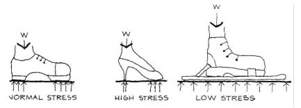
Normal shoes cause normal stresses and can be used on surfaces that can resist these stresses. High heeled shoes, as they provide a much smaller area to carry the same weight, cause higher stresses under the shoe, particularly under the heel. Where stresses must be kept low, for walking on snow for instance, the area under the foot must be increased. This is why snowshoes prevent people from sinking into snow.
