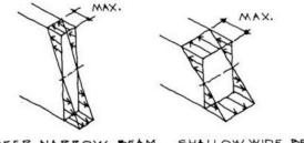
Beams bent by moments have varying stresses that are at a maximum at the top and bottom. As all structural materials have a maximum usable stress, rectangular solid beams are understressed except for the top and bottom faces.
