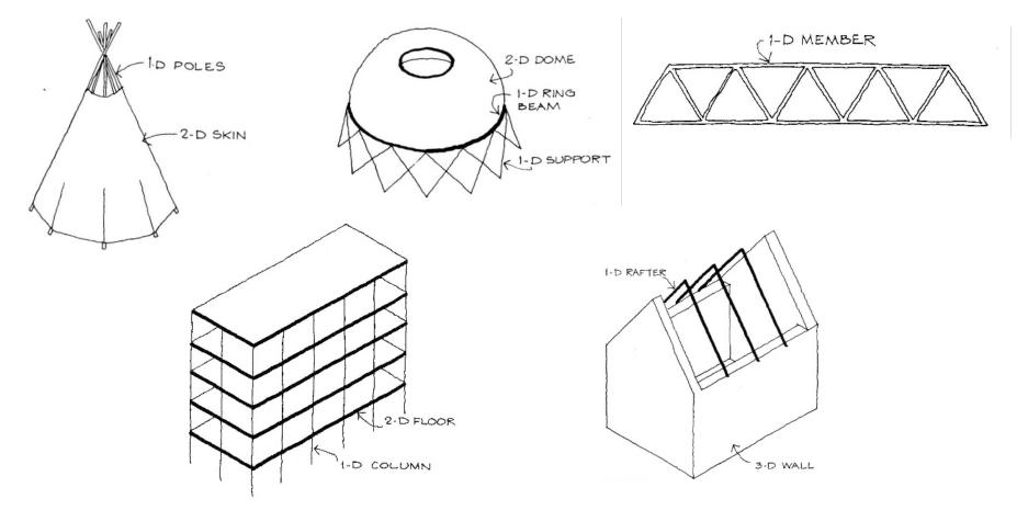
Nowadays structures are usually conceived and designed as assemblies of structural elements. This means the structural behaviour can be identified by considering the behaviour of each **structural element** in each load path.
